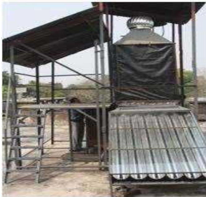
Figure 8.11 : Solar-biomass Integrated Drying System for Spices
